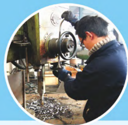
立式镗铣床 Horizontal Boring And Milling Machine
