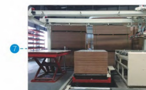
移栽机堆垛 Vacuum stocking system
