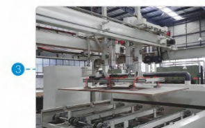
吸盘移栽机构 Vacuum transfer system
